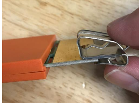
Figure 8: CC-TC clip insertion at flush side for clip-mount
